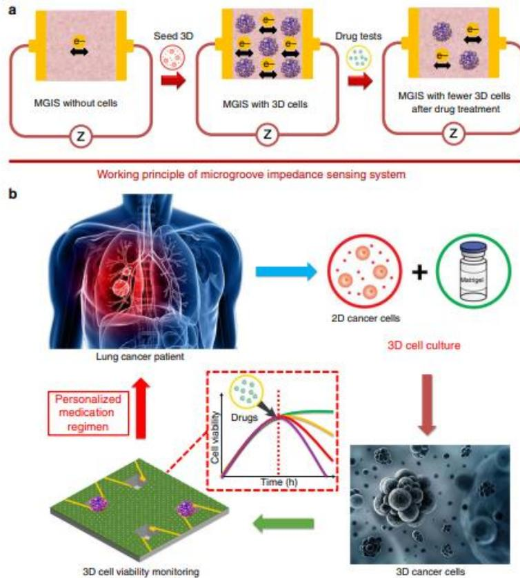
**Figure 2** Schematic illustration of 3D cell sensing and detection. **a** The working principle of 3D ECIS: the number of living cells influences the conductivity of the Matrigel/cell construct. **b** Schematic of the 3D ECIS for antineoplastic drug screening (Adapted from Ref. [14]).
